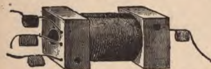
FIG. 42.—Induction Coil of the type used in telephones.
